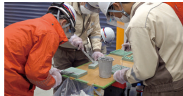
Practical training on preparing organic material test specimens (resin adhesives)
