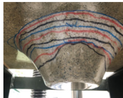
Transparent spalling prevention using single-component urethane resin
