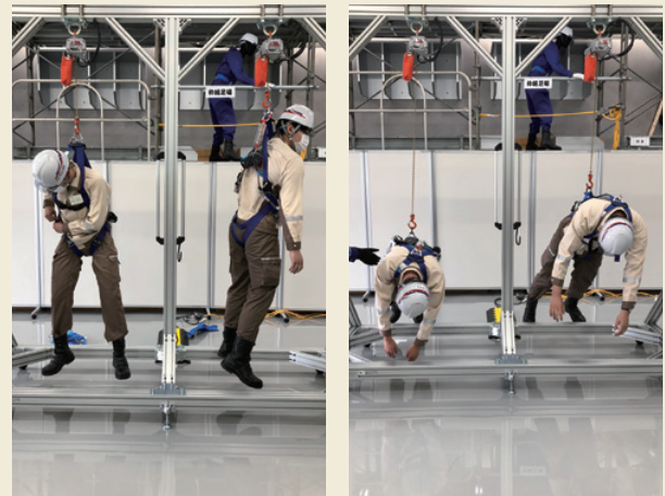
Training participants are suspended by a harness (left) and torso belt (right).
