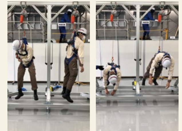
Training participants are suspended by a harness (left) and torso belt (right).
