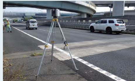
Structure measurement using a 3D scanner
