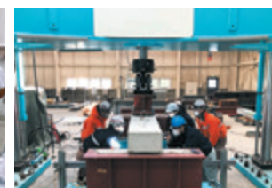
Bending test of deck slabs repaired by resin injection
