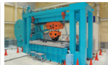
Wheel load running test
