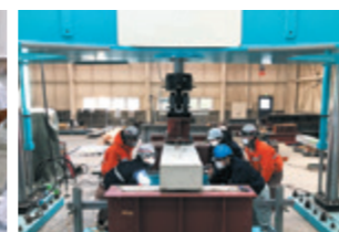
Bending test of deck slabs repaired by resin injection
